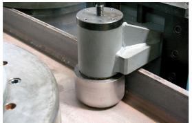
MAH600/3AC Electronic overload protection Hydraulic angle bending guide rolls
